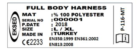
Above label contains Brand name (EKSED), Indication of conformity with the directive (CE2233), Number of the standard to which the product conforms (EN 361), Product reference (P-115-MT), Serial number (000001), Material(100%polyester), Size(L/XL), Read the instruction before use.
